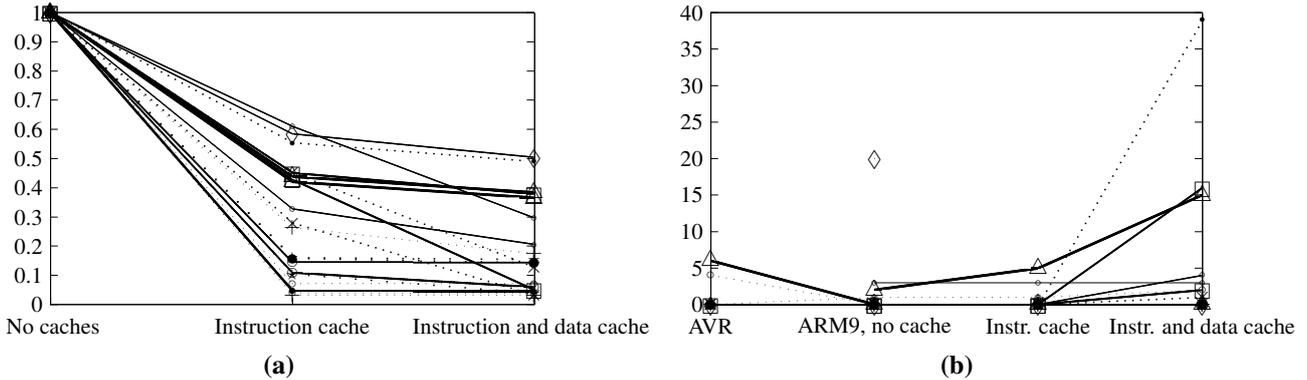
**Figure 6.** (a) Improvement in WCET estimate by precisely modelling the different caches on the ARM9. The average improvement in WCET estimate is 71.6% by modelling the instruction cache, and 81.3% by modelling both caches. (b) Analysis times for the different configurations in minutes. The average succesful analysis times are, respectively: 52.46 secs., 83.61 secs., 44.8 secs. and 265.75 secs.
